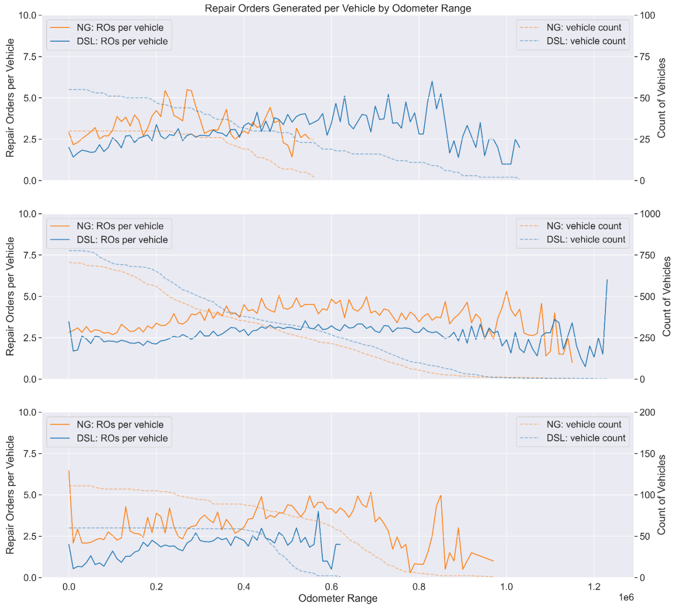
Figure 21: Average Number of ROs Generated per Active Vehicle by Fleet and Fuel Type (Fleet 0 is shown in the topmost graph, followed by Fleet 1 and Fleet 2.)
